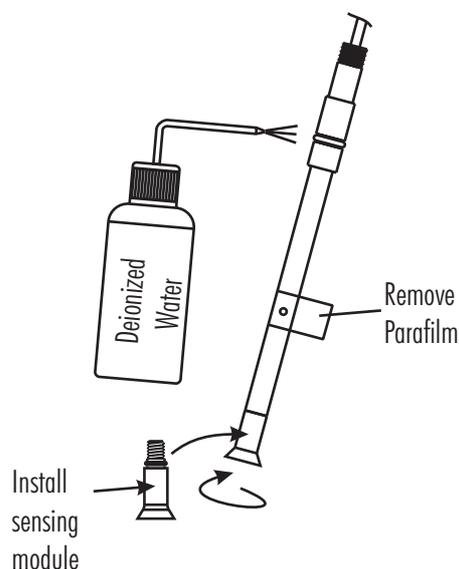
6. Reassemble electrode by gently pushing the inner assembly into the outer body, sliding spring down cable, and screwing cap into place. **DO NOT TOUCH OR PUT PRESSURE ON LANTHANUM CRYSTAL.**
