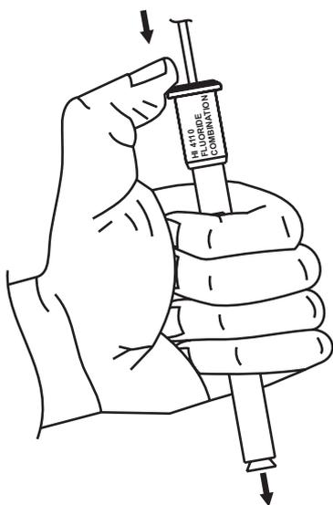
10. Tighten the electrode cap onto the body and fill electrode body until fill solution volume is just below fill hole.
