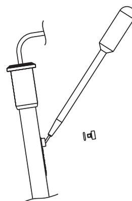
9. Holding the body of the electrode gently press upper cap with your thumb. This permits the fill solution to drain out of the body. Release cap and verify electrode returns to its original position (you may need to gently assist for this to occur).
